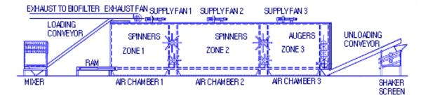
Each zone has its own air supply and a biofilter exhaust fan to minimize odor. The configuration of airflow and temperatures kills the pathogens in a 14-day cycle and the material then comes out of the machine. The product must then be stockpiled to cure for another 30 to 90 days, depending upon the quality of compost desired.
